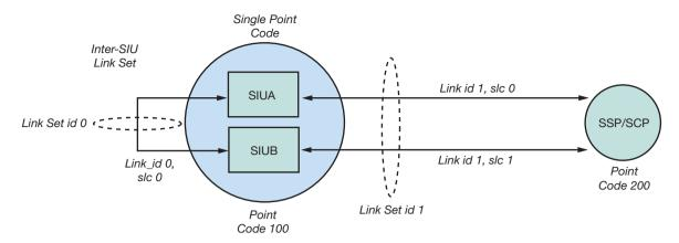
Figure 19. Example Configuration to an Adjacent SSP/SCP
